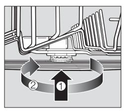
■ Lift up the <u>middle</u> spray arm, ①, to engage the ratchet and unscrew the spray arm, ②.
